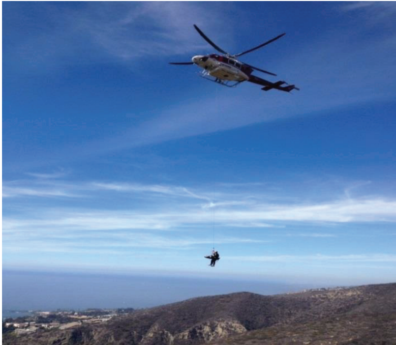
Figure 4 OCFA helicopter using hoists
