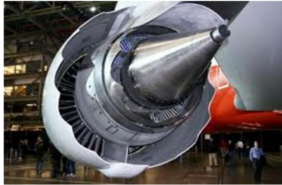
Photograph: Nacelle Chevron
