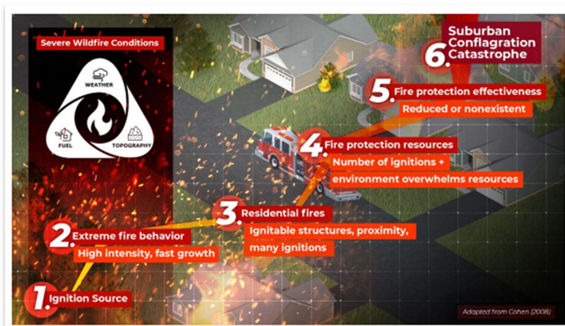
Figure 3 WUI and suburban conflagration fire disaster chain of events. 21
